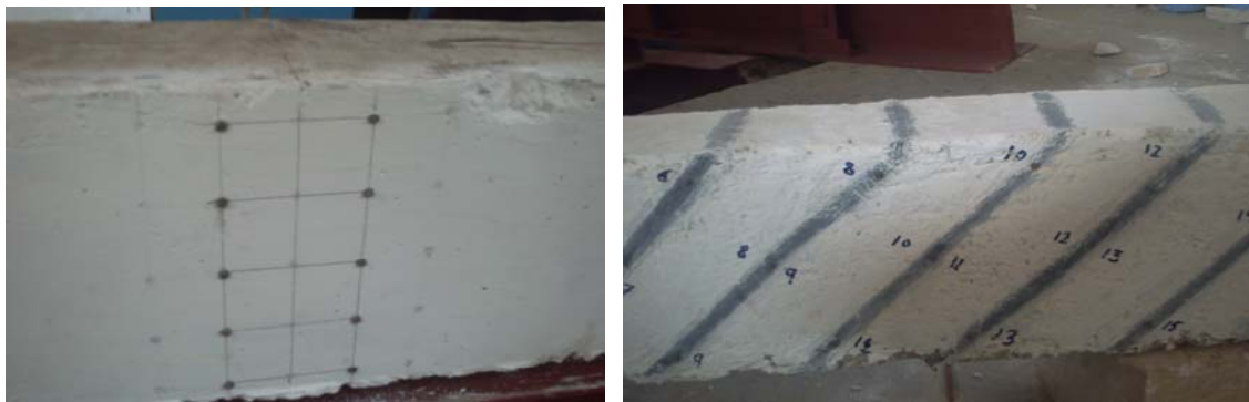
FIGURE 5, Demec Points in Concrete and CFRP
